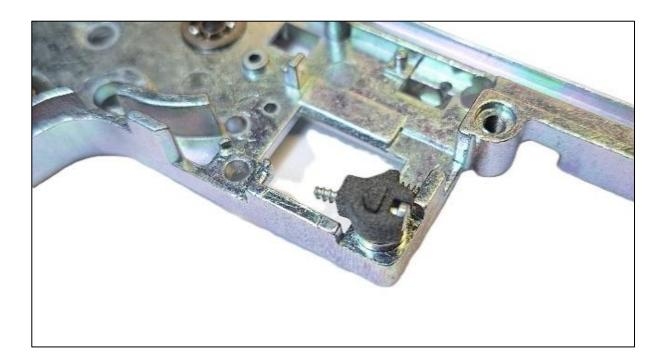
Do not turn the screw all the way in, the head should remain around a millimeter away from the hole. Put the gearbox halves together only with the main body of the Clicker and the lock inside, and while looking through the selector window, adjust the screw so, that while on SAFE the tip of the screw will be touching the metal part of the Clicker, yet it will still be able to engage and disengage freely while
