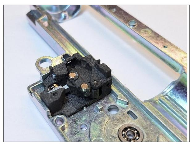
Clicker V2 PRO comes with its own mechanical trigger lock. The main part of the lock has to fit well into the shell's corresponding hole, therefore 6 pieces with varying dimensions are provided, where 1 is the thinnest and 6 is the thickest. Choose the one, which will be the most stable inside the hole, while at the same time allowing the return spring to disengage the lock when the selector is not set to "SAFE".
