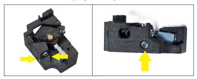
Limiting the overtravel too much will cause the trigger not to reset properly, i. e. further shots will not be fired immediately after the trigger resets with an audible click. If the replica does not fire another shot unless the finger is taken completely off the trigger, increase the amount of overtravel.
