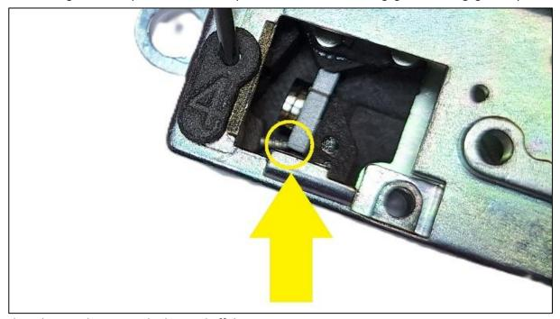
the selector is being switched on and off the SAFE position.
