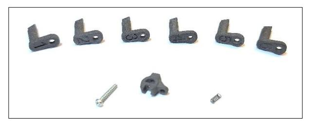
To accommodate various gearbox shells and selector plates, the main part of the lock purposefully made too long in the area where it touches the selector plate, and in some replicas it might block the trigger already on SEMI selector position. If needed, grind down or carefully cut the part a bit to adjust it to the replica and selector plate in question.
